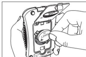
**Note:** after the battery is replaced, the meter displays the “all segments” screen. Then, the meter displays the time set up. Reset to the current time and date. If needed, go to Paragraph 4 at page 20 in this guide to review setting the time, date, markers, and beeper.
