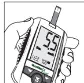
**Note:** if test result is above 8.0 mmol/L for  $\beta$ -ketone, the screen displays HI with Ket displaying.
