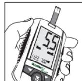
**Note:** if test result is above 33.3 mmol/L, the screen displays HI; if test result is below 1.1 mmol/L, the screen displays LO.
