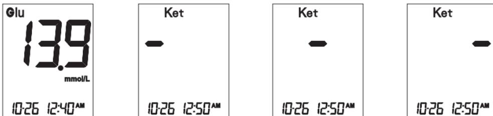
**Note:** when in this display cycle, pressing ANY key will 'freeze' the display showing the glucose value. The user can then use the Left/Right buttons to toggle between marking and unmarking a test result.
